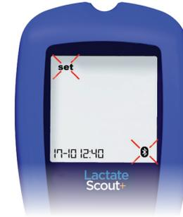
After pressing the scroll wheel briefly, the menu is activated and the message "OFF" is displayed on the main display together with the blinking Bluetooth® icon:
