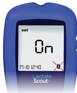
After pressing the scroll wheel briefly, the Bluetooth® module is activated. Please note: The device will turn off automatically after five minutes if no user input is detected. However, you can turn on the device again as already described above and continue working. (See Lactate Scout+ manual).
