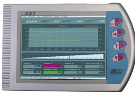
Fig. 20: Heart rate monitoring is a basic feature of many ergometers - the Cyclus 2 offers additionally a data interface to lactate analyzers
