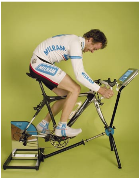
Fig. 28: The CYCLUS 2 converts the own bike into a very individual and very professional ergometer
